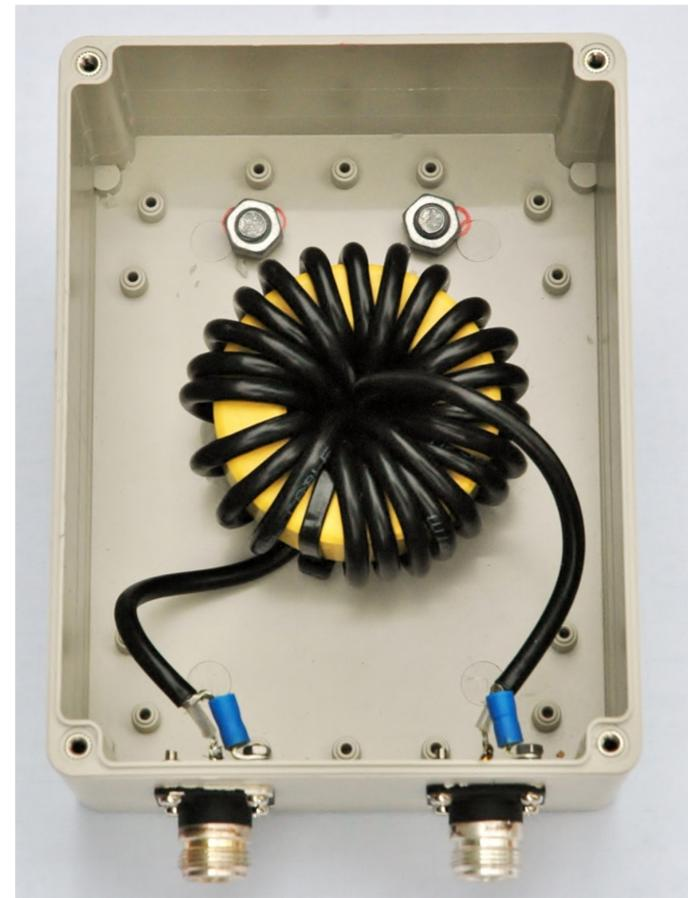
Photo 1 Low band choking balun assembled.
