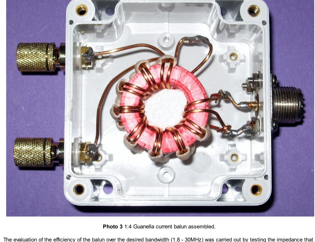
could be seen from unbalanced side to a resistive load applied to the balanced side using an antenna analyser. The efficiency is shown to be relatively flat from below 1.8MHz to above 30MHz. The below antenna analyser plot viewing a 200ohm resistive load
