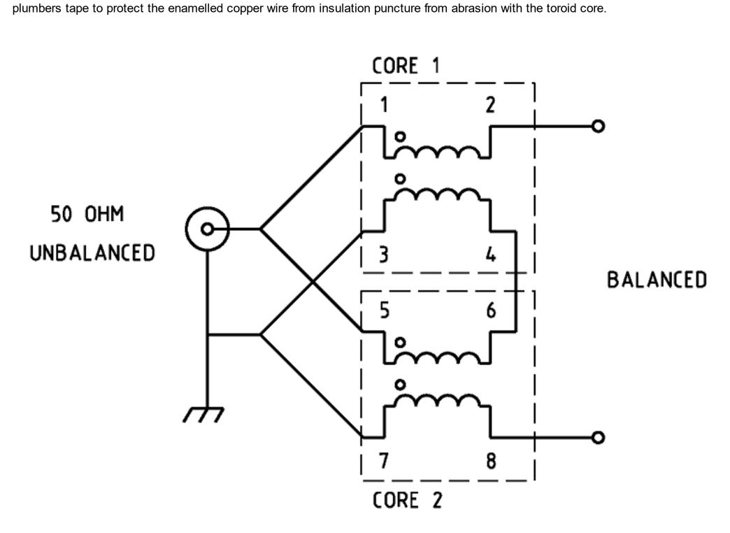
Figure 1 Schematic of the 1:4 Guanella Current balun.
