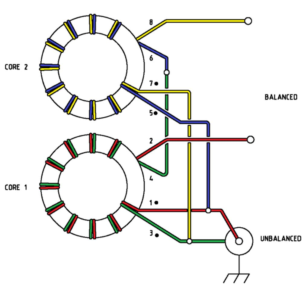
Figure 2 Wiring of the 1:4 Guanella Current balun. Note this drawing shows winding connections and not the number of turns required. See article for details.
