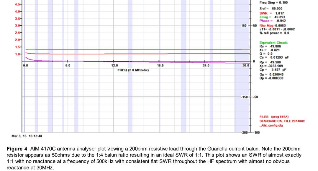
Zmag Rs,Xs Phase Min SWR = 1.87 @ 29.900 MHz 300 100 Freq = 0.607
