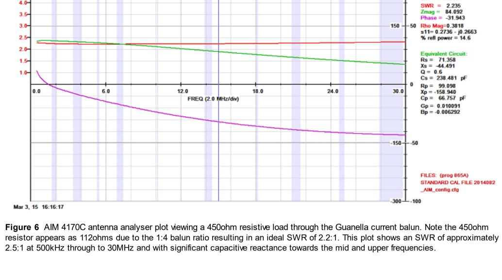
AIM 4170C antenna analyser explanation; SWR Standing Wave Ratio.
