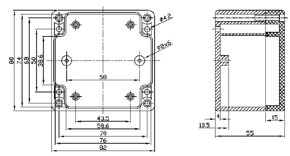
Figure 3 Sealed Polycarbonate Enclosures 82 x 80 x 55mm details. Designed to IP65 of IEC 529 and NEMA 4
