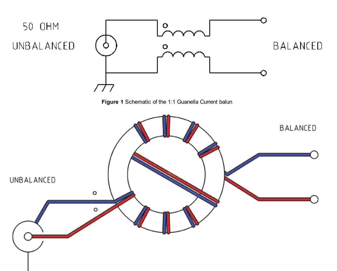
Note this drawing shows winding connections only and not the number of turns required. See article for details.
