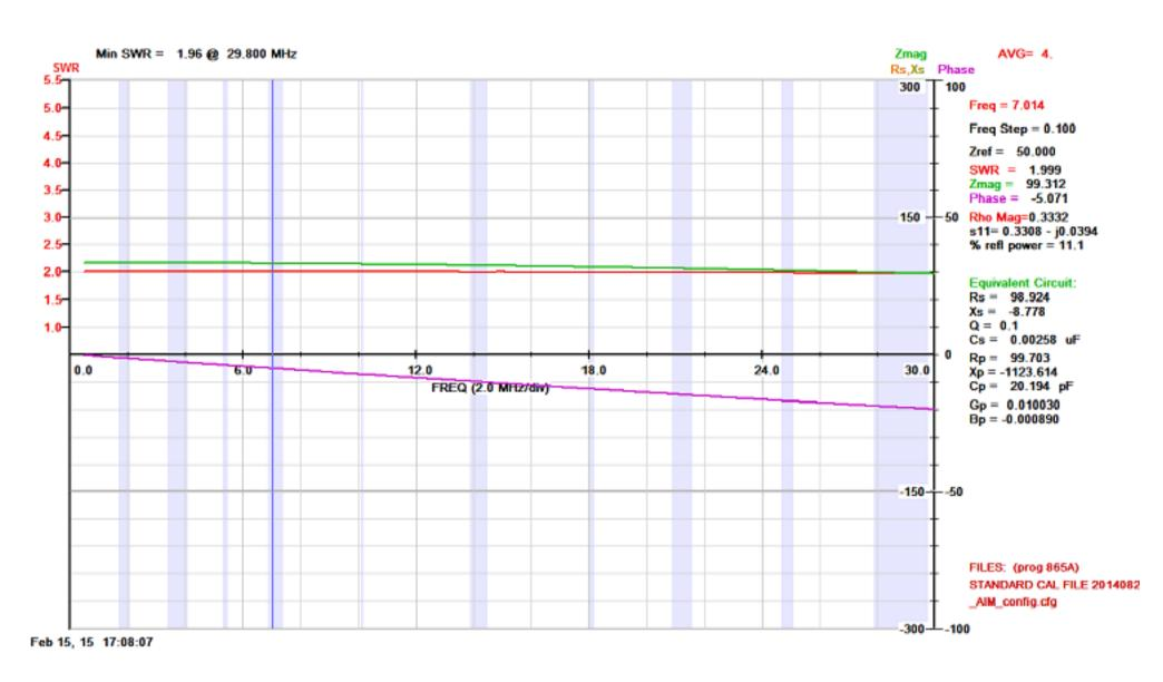
**Figure 5** AIM 4170C antenna analyser plot viewing a 100ohm resistive load through the Guanella current balun. Note the 100ohm resistor appears as 100ohms due to the 1:1 balun ratio resulting in an ideal SWR of 2:1. This plot shows an SWR of approximately 2:1 from 500kHz through to 30MHz and with modest capacitive reactance towards the upper frequencies.
