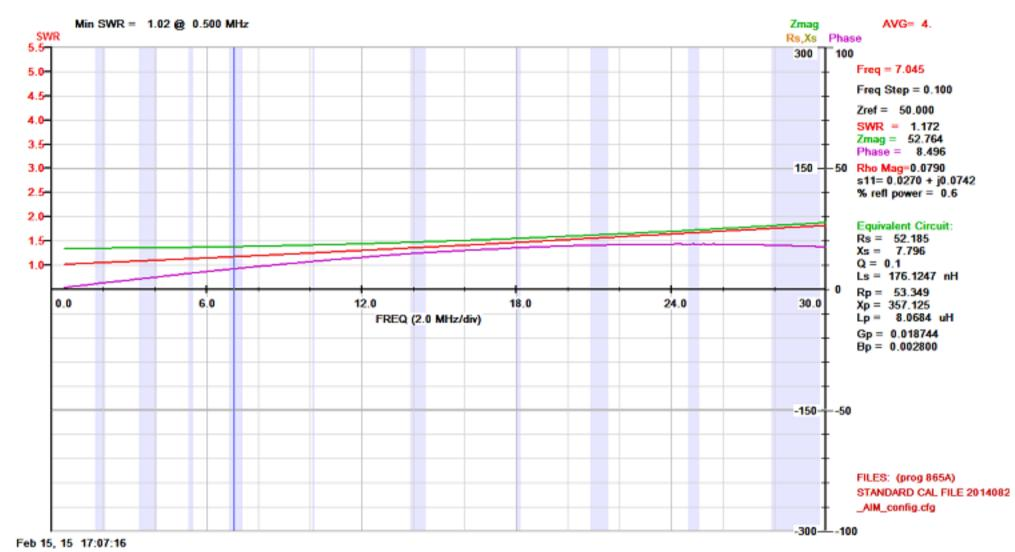
**Figure 4** AIM 4170C antenna analyser plot viewing a 50ohm resistive load through the Guanella current balun. Note the 50ohm resistor appears as 50ohms due to the 1:1 balun ratio resulting in an ideal SWR of 1:1. This plot shows an SWR of almost exactly 1:1 with no reactance at a frequency of 500kHz with consistent rise in SWR throughout the HF spectrum to an SWR of approximately 1.8:1 and some inductive reactance at 30MHz.
