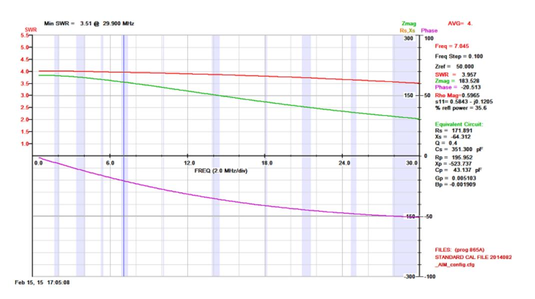
**Figure 6** AIM 4170C antenna analyser plot viewing a 200ohm resistive load through the Guanella current balun. Note the 200ohm resistor appears as 200ohms due to the 1:1 balun ratio resulting in an ideal SWR of 4:1. This plot shows an SWR of approximately 4:1 at 500kHz dropping to approximately 2:1 at 30MHz and with significant capacitive reactance towards the mid and upper frequencies.
