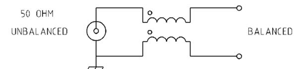
Figure 1 Schematic of the 1:1 Guanella Current balun
