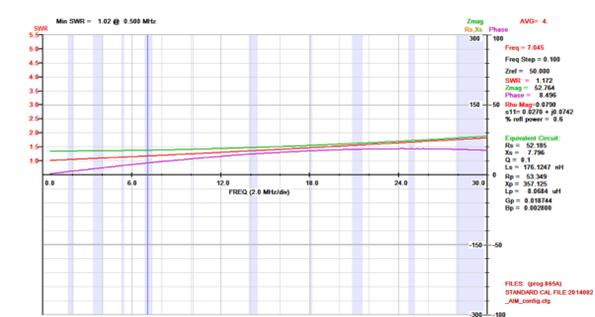
Figure 4 AIM 4170C antenna analyser plot viewing a 50ohm resistive load through the Guanella current balun. Note the 50ohm resistor appears as 50ohms due to the 1:1 balun ratio resulting in an ideal SWR of 1:1. This plot shows an SWR of almost exactly 1:1 with no reactance at a frequency of 500kHz with consistent rise in SWR throughout the HF spectrum to an SWR of approximately 1.8:1 and some inductive reactance at 30MHz.
