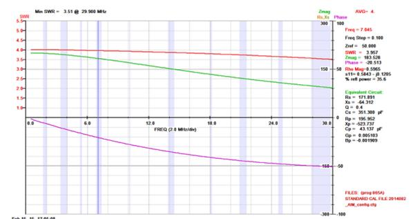
Figure 6 AIM 4170C antenna analyser plot viewing a 200ohm resistive load through the Guanella current balun. Note the 200ohm resistor appears as 200ohms due to the 1:1 balun ratio resulting in an ideal SWR of 4:1. This plot shows an SWR of approximately 4:1 at 500kHz dropping to 2:1 at 30MHz and with significant capacitive reactance towards the mid and upper frequencies.
