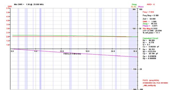
Figure 5 AIM 4170C antenna analyser plot viewing a 100ohm resistive load through the Guanella current balun. Note the 100ohm resistor appears as 100ohms due to the 1:1 balun ratio resulting in an ideal SWR of 2:1. This plot shows an SWR of approximately 2:1 from 500kHz through to 30MHz and with modest capacitive reactance towards the upper frequencies.
