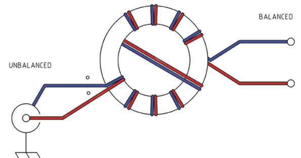
Figure 2 Wiring of the 1:1 Guanella Current balun.
