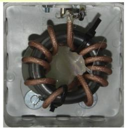
The 400-Watt Current Balun with a FT140-43 core and 2x5turns of PTFE-coax cable
