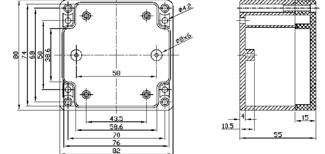
Figure 4 Sealed Polycarbonate Enclosures 82 x 80 x 55mm details
