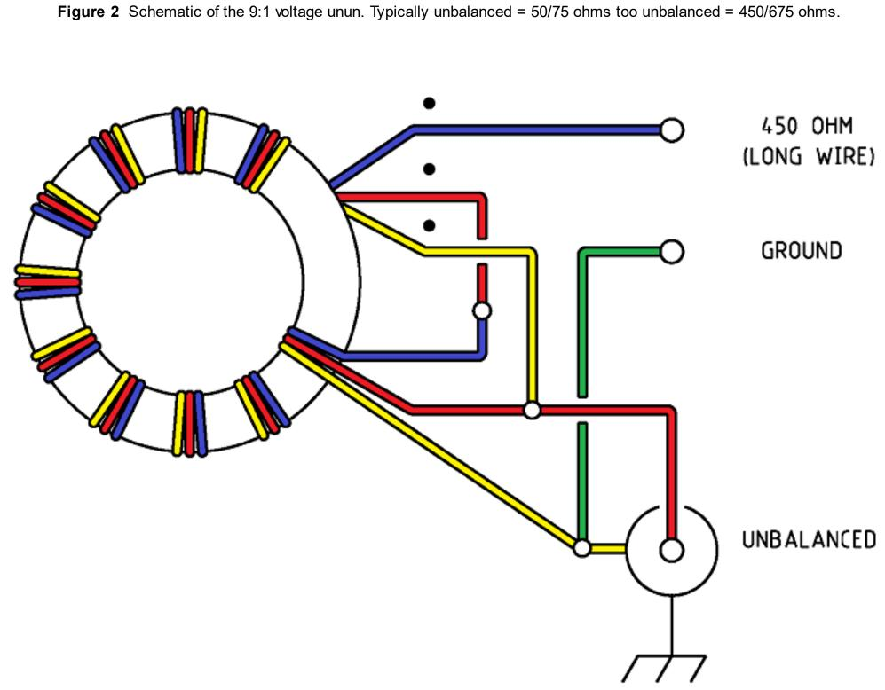
Figure 3 Wiring of the 9:1 voltage unun. Note this drawing shows winding connections and not the number of turns required. See article for details.
