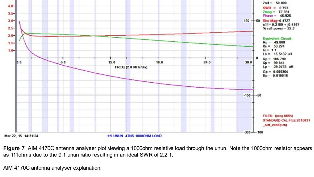
SWR Standing Wave Ratio. Total Impedance. **Z**mag
