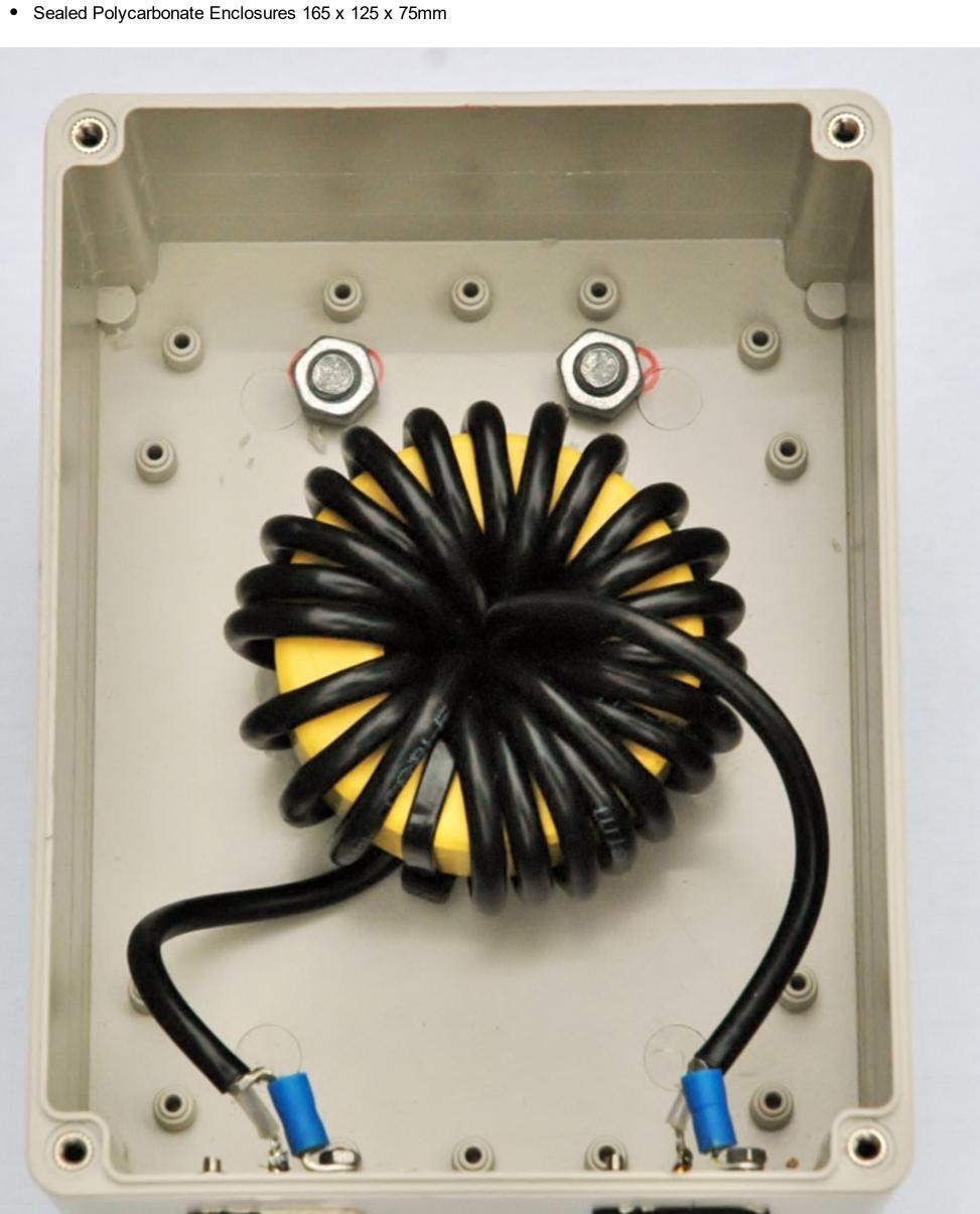
Photo 1 Low band choking balun assembled.
