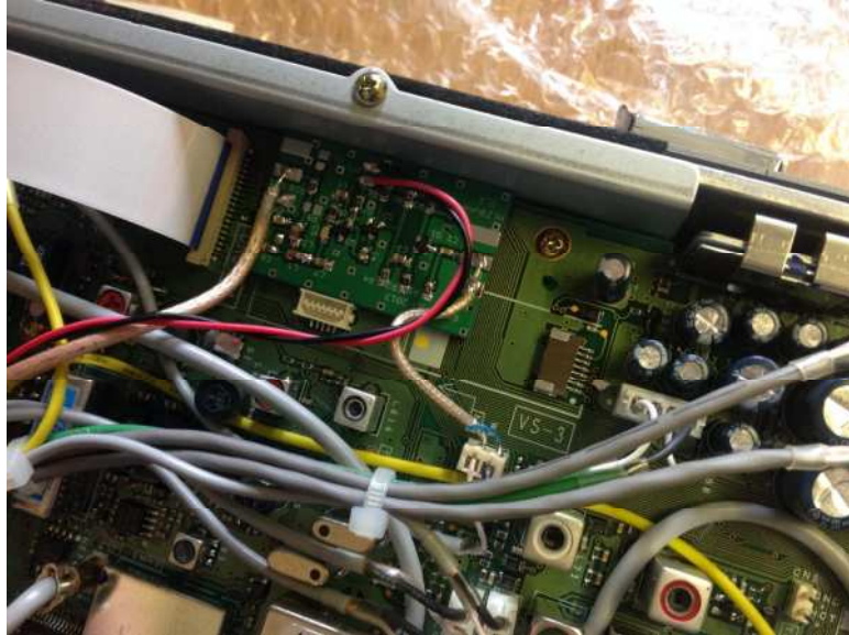
Fig 4 - PAT installed in TS2000
