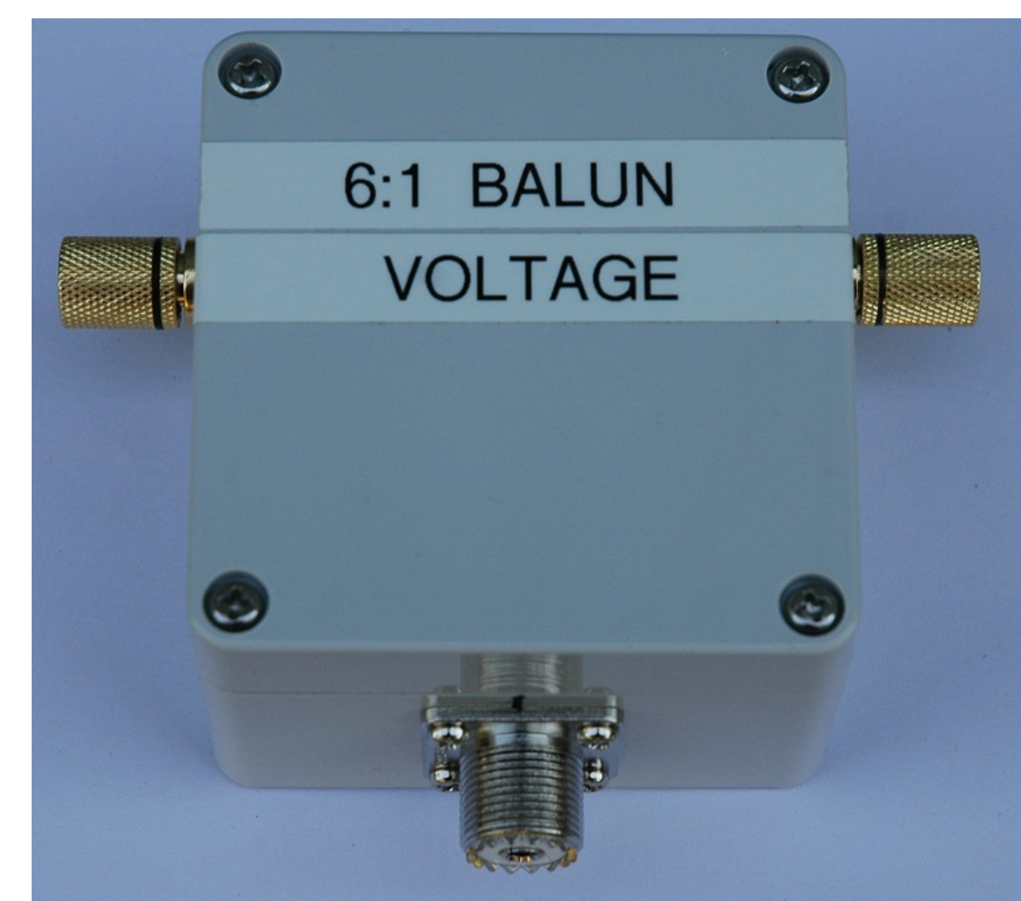
Photo 3 1:6 Voltage balun assembled in weatherproof enclosure.
