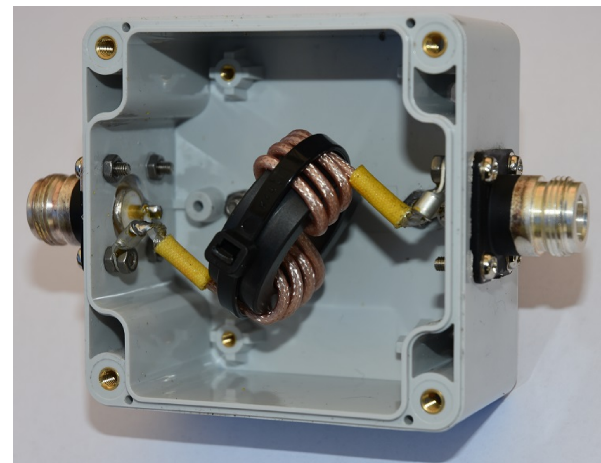
Photo 1 Low band choking balun assembled.
