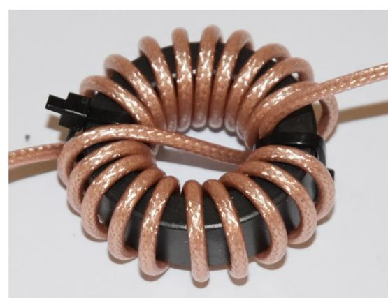
Photo 1 Choking balun assembled.
