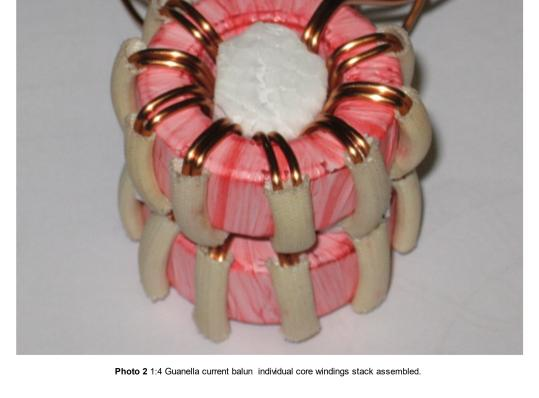
Photo 2 1:4 Guanella current balun individual core windings stack assembled.
