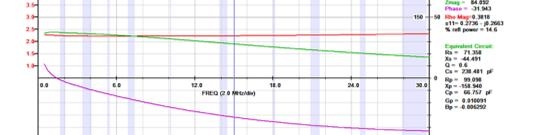
Figure 6 AIM 4170C antenna analyser plot viewing a 450ohm resistive load through the Guanella current balun. Note the 450ohm resistor appears as 112ohms due to the 1:4 balun ratio resulting in an ideal SWR of 2.2:1. This plot shows an SWR of approximately 2.5:1 at 500kHz through to 30MHz and with significant capacitive reactance towards the mid and upper frequencies.
