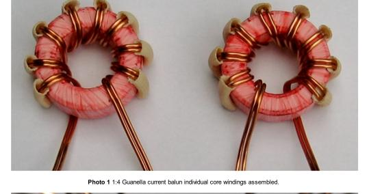
Photo 1 1:4 Guanella current balun individual core windings assembled.
