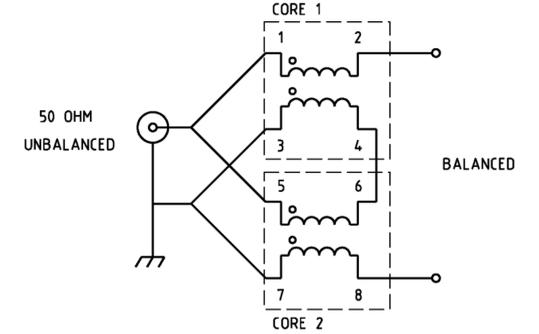
Figure 1 Schematic of the 1:4 Guanella Current balun.
