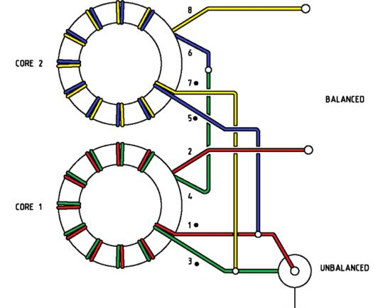
Figure 2 Wiring of the 1:4 Guanella Current balun.
