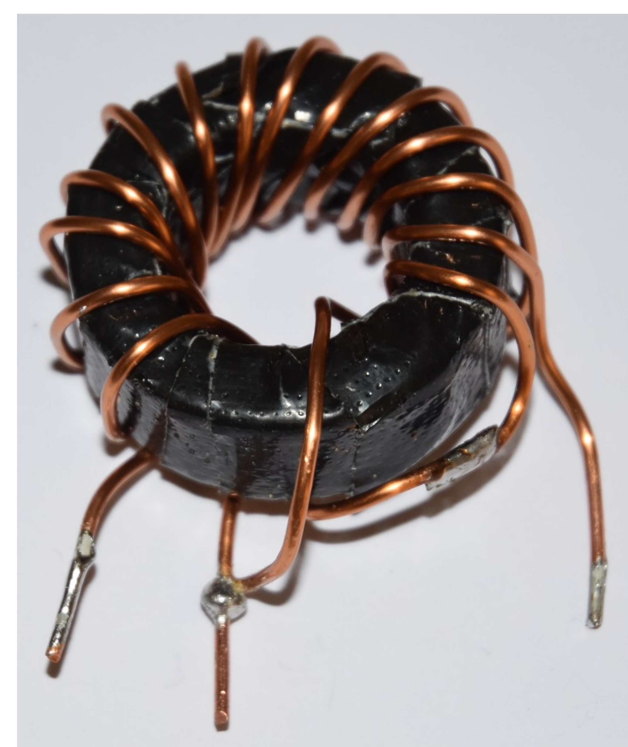
Photo 1 Completed core winding assembly. note fibre glass tube sections to hold winding groups together.
