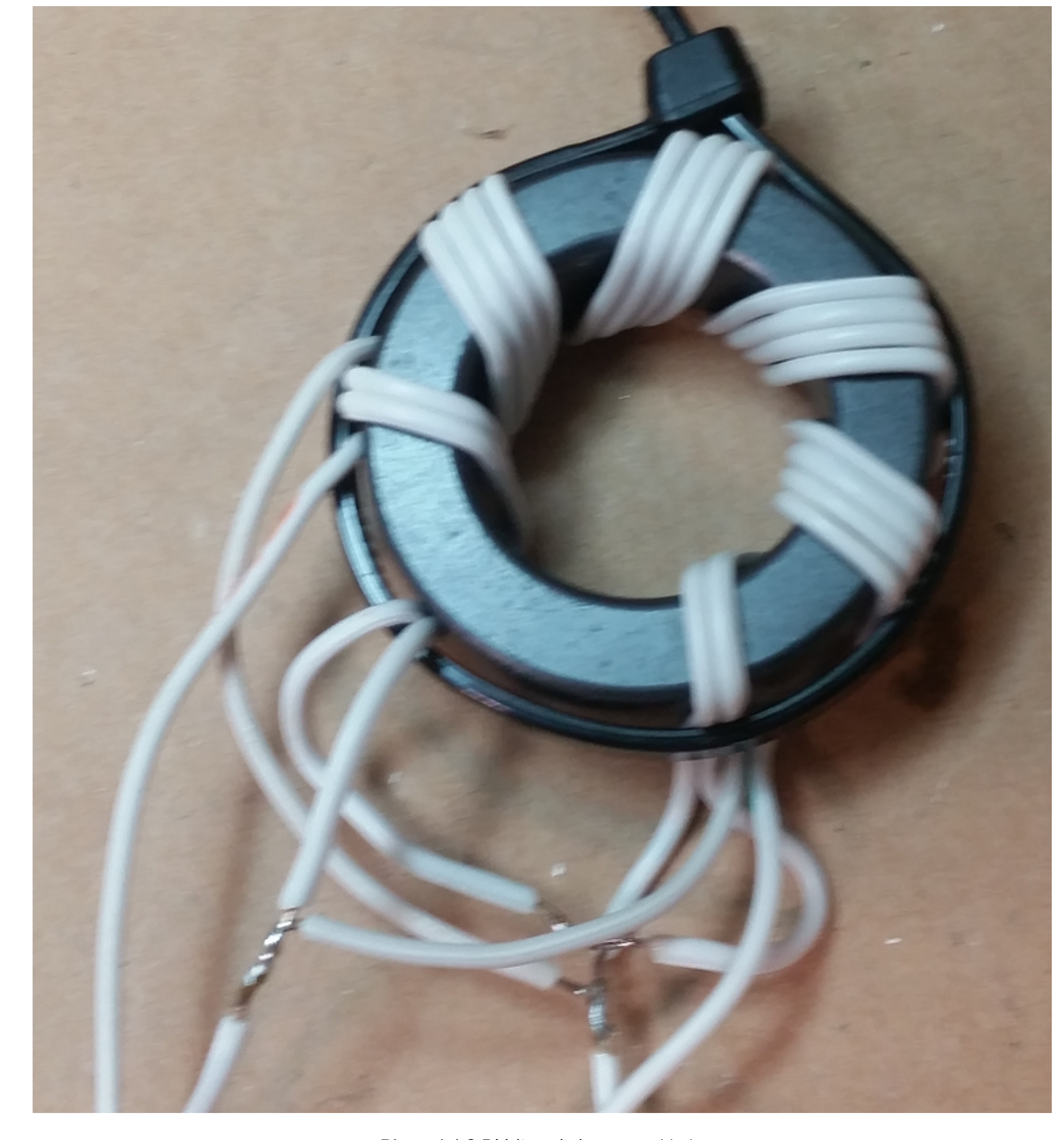
Photo 1 1:2.5 Voltage balun assembled.
