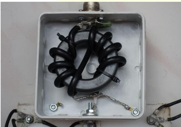
The 1KW-Current Balun with a FT240-43 core and 2x4 turns Aircell-5
