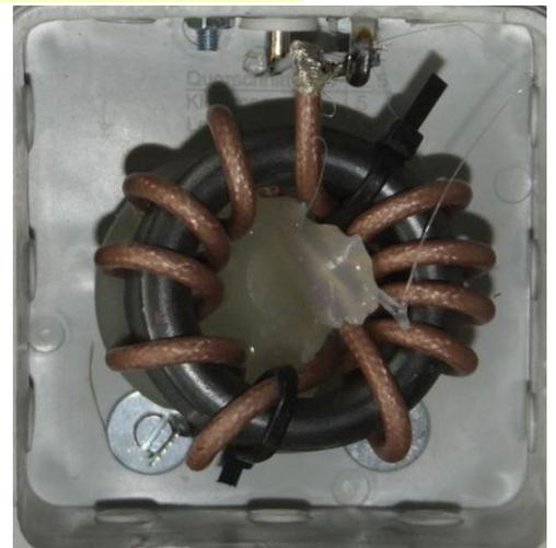
The 400-Watt Current Balun with a FT140-43 core and 2x5turns of PTFE-coax cable
